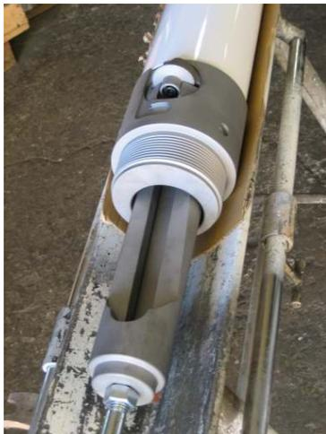
Push the slide up and down to make sure it slides easily and the cutter blade goes in and out.
