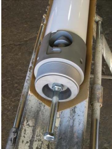
These parts should be oiled (Rock Drill oil works well).
