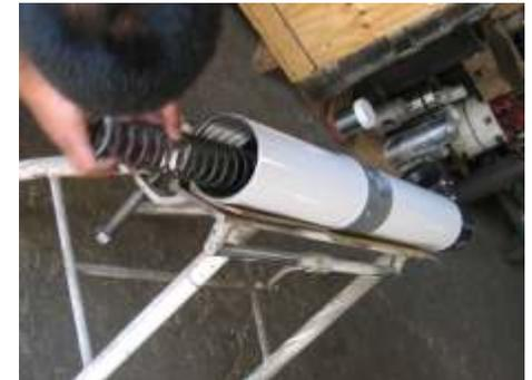
It may take two strong people to push the spring in and start threading the **Bottom Cap #16**. To change the blade, unscrew the Bottom Cap far enough to allow the **Vertical Slide #12** to be pushed down by air (or by broom stick) allowing the cross slide to be pulled out.
