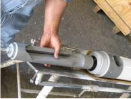
Insert **Vertical Slide #12** from the bottom.
