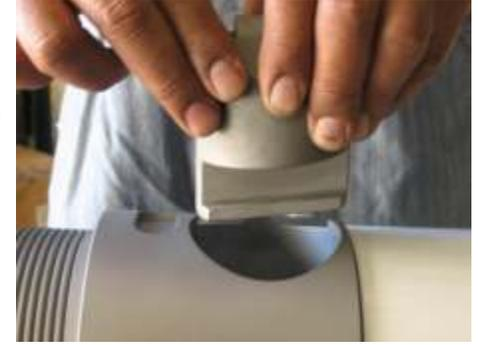
Push the **Vertical Slide #12** upward and trap the Blade Holder Cross Slide #8 in the T-slot track.
