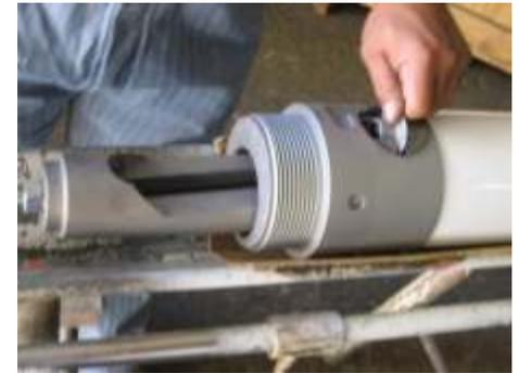
The **Stroke Adjustment Bolt #14** is pre-adjusted and locked by the **Locking Nut #13** at the factory.
