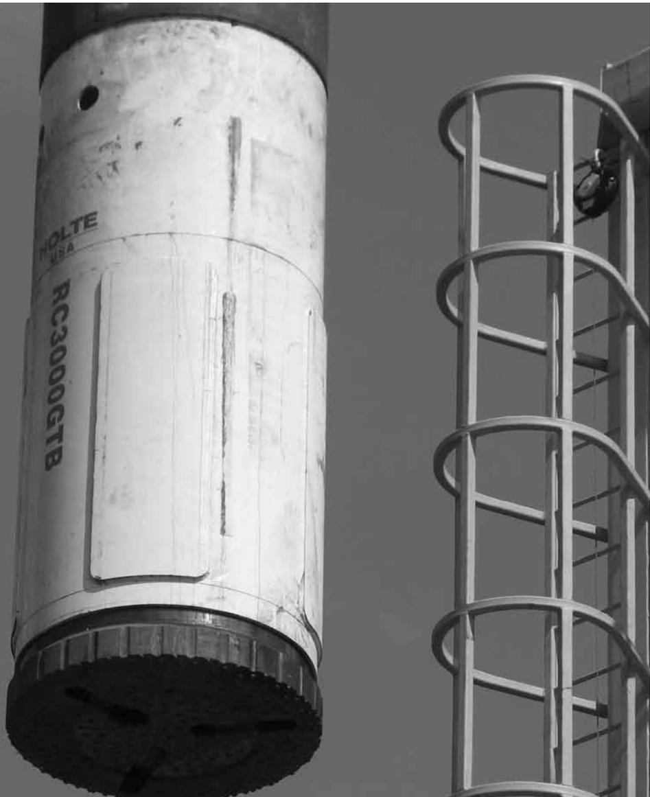
**REVERSE CIRCULATION DOWN HOLE HAMMERS [ RCDHH ]**
