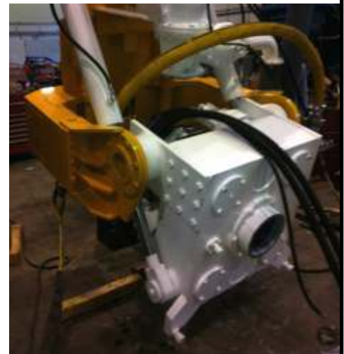
Drive head later mounted on a Bauer RTG 21 sled operating in France.
