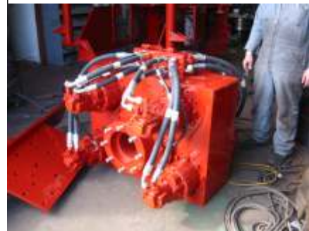
Reverse circulation (RC) TOP HEAD DRIVE with swivel and discharge elbow.
